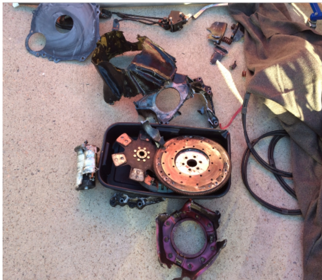
The carnage from Steve's exploded clutch.
